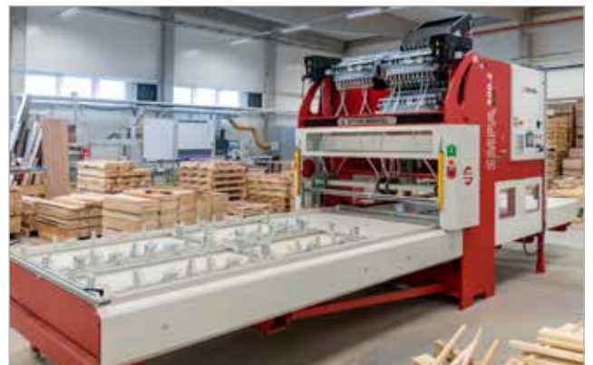
Stacking machine for the production of pallets
